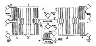
Symmetric Beam Width Compression Multistrip Coupler
