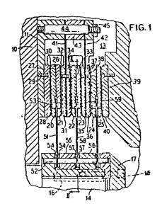
The present invention is directed to a refining apparatus of the type used in the treatment of fibrous suspensions in paper making and involves a flexible link interconnection between a rotary drive means and refiner disks which provide the refining action.
