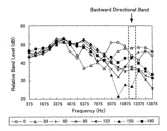
Rising angle indicative of sound source position with front direction of median plane being zero degree
