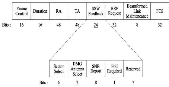
11ad SSW-Feedback frame & SSW-ACK frame
