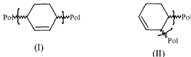
35 The 1,4- to 1,2- relative ratio can be modified by varying the catalyst and reaction conditions. In embodiments, the PCHD comprises 1,4-addition units and 1,2-addition units of CHD in a relative mole ratio of 90:10 to 10:90, or 50:50, or 30:70 to 70:30, or 40:60 to 60:40, or 20:80 to 80:20.
