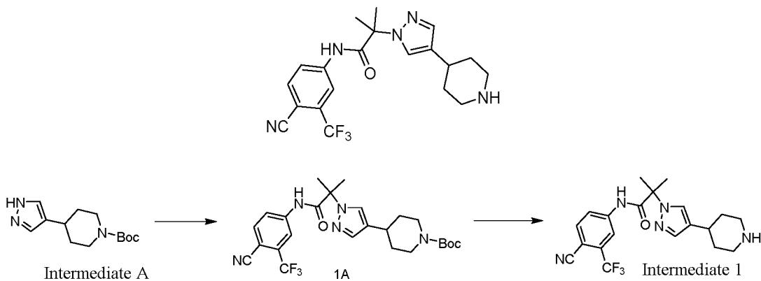
Step 1: tert-butyl 4-(1-(1-((4-cyano-3-(trifluoromethyl)phenyl)amino)-2-methyl-1-oxopropan-2-yl)-1H-pyrazol-4-yl)piperidine-1-carboxylate (1A)
