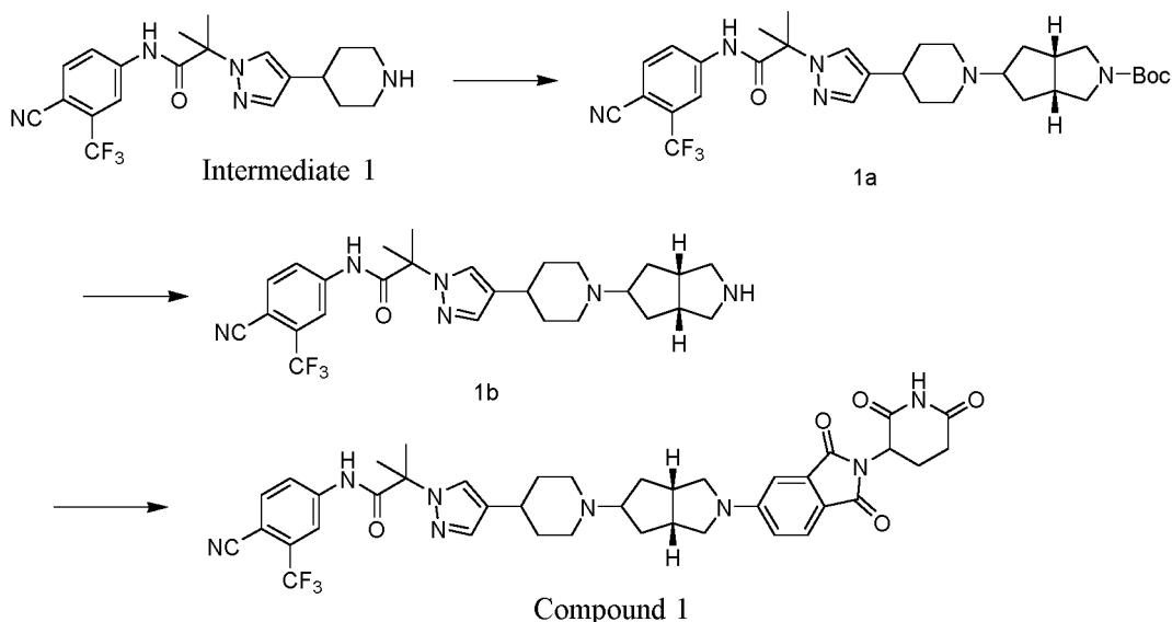
Step 1: tert-butyl(3aR,6aS)-5-(4-(1-(1-((4-cyano-3-(trifluoromethyl)phenyl)amino)-2-methyl-1-oxopropan-2-yl)-1H-pyrazol-4-yl)piperidin-1-yl)hexahydrocyclopenta[c]pyrrole-2(1H)-carboxylate (1a)
