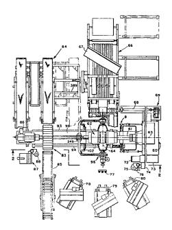
thus the tire being built. A bead gripper, actuated by fluid power, automatically rotates clear of the bead flippers or apex and clamps the tire bead securely and squarely to ensure accurate bead placement while transferring the tire bead to its selected location. A retractable positive inter-
