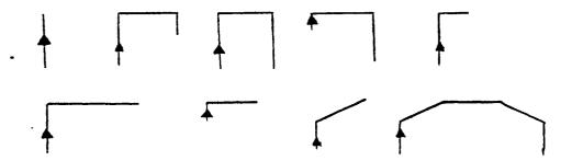
The illustrated nine shapes, along with the conjugates of the second to the ninth shapes; provide a set of seventeen selected canonic shapes which are later matched against the character curve segments of the character being scanned so that a "best match" can be determined and used in the recognition process.
