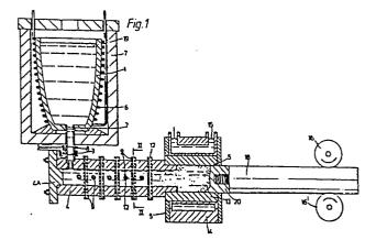
The present invention relates to an apparatus and posses for cooling a flow of a molten material which is to be directed to a means for casting the material.
