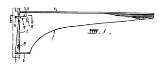
This invention relates to a shelving system of the type in which the shelves are supported on brackets located in position on elongated upright members. In particular, this invention relates to an improved shelving bracket for such a shelving system.
