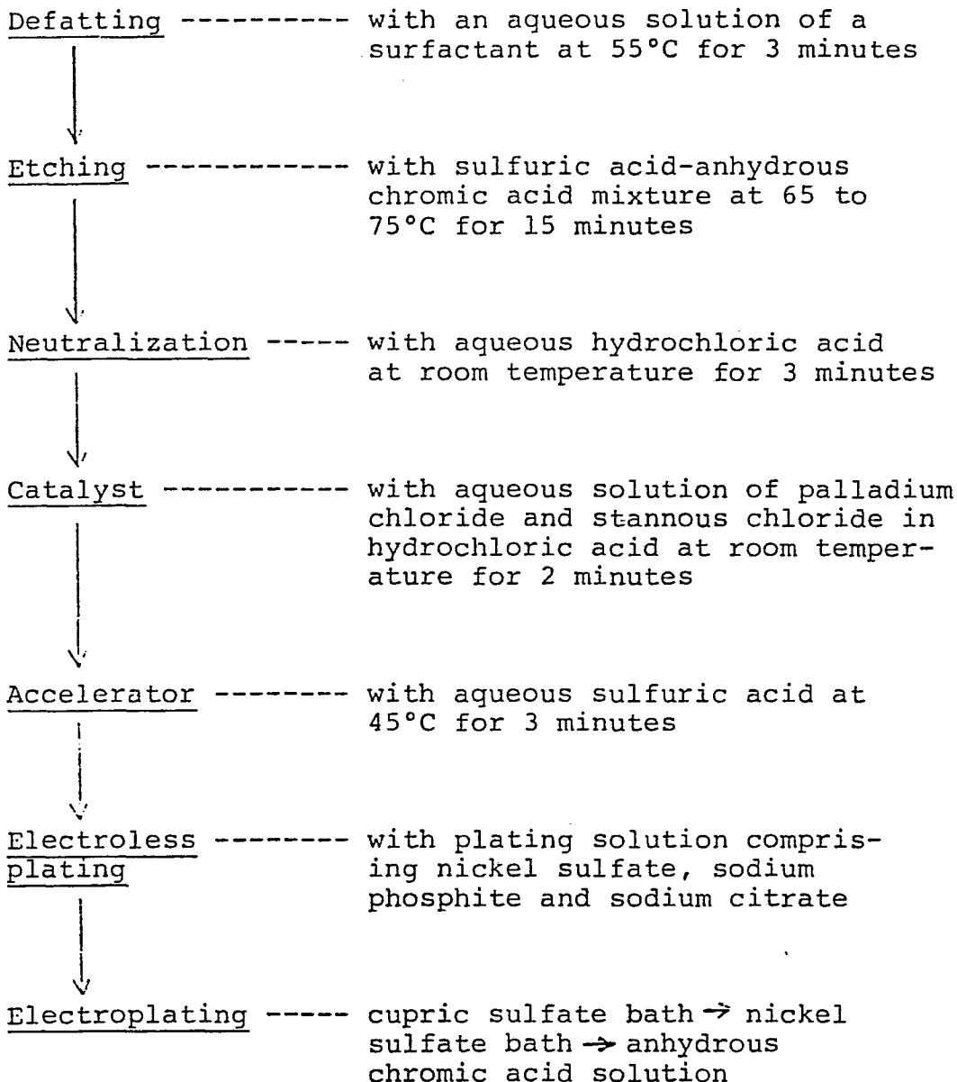
In the above typical plating procedure, a copper film and then a nickel film are formed on the surface of the molded product. In order to enhance the corrosion resistance, the cupric sulfate bath is often replaced by one nickel sulfate bath or two nickel sulfate bathes. In such case, double nickel plating or triple nickel plating is effected. Usually, the thus double nickel plated or triple
