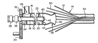
This invention relates to the production of multi-stranded electrical cables and more particularly to filling the interstices of such cables.
