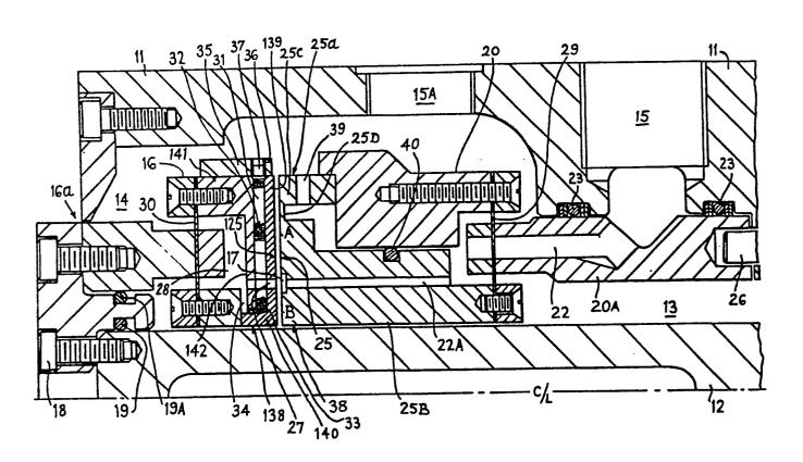
"MEANS FOR COOLING MECHANICAL WORKING ELEMENTS, SUCH AS BEARINGS, RADIAL FACE SEALS OR FRICTION DEVICES"
