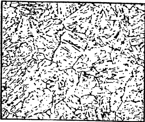
(c) Bainite starting structure (Mo-Cr steel)
