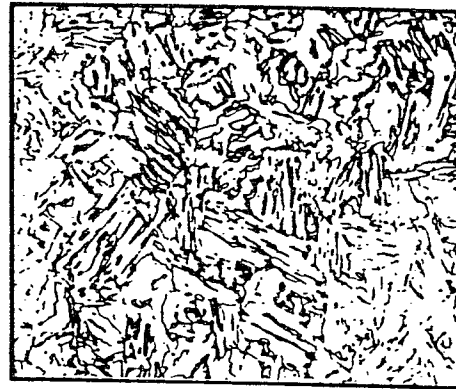
(d) Typical dual-phase structure resulting from (c)
