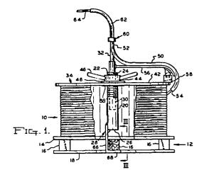
Dispenser for filamentary material, especially welding wire.
