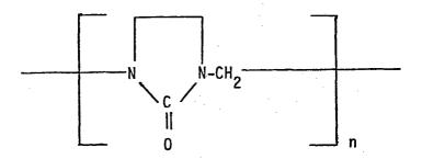
wherein n is an integer from 20 to 60 having a mean value of 41, and by an average number molecular weight  $\rm M_n$  ranging from 2000 to 6000.
