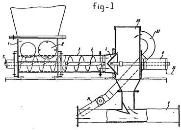
A metering device for powdery material, in particular powdery fuel.
