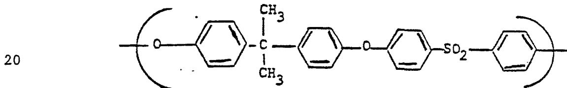
The polyarylene polyether polymers are prepared by the procedures as set forth in U.S. Patents 4,108,837 and 4,175,175, i.e., by the substantially equimolar reaction of a double alkali metal salt of a dihydric phenol with a dihalobenzenoid compound in the presence of liquid organic sulfone or sulfoxide solvents and co-solvents under substantially anhydrous conditions.
