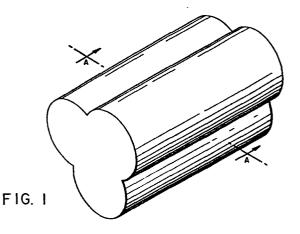
The present invention relates generally to adsorption processes utilizing agglomerated bodies of crystalline zeolitic molecular sieves, and more particularly to improved large-scale adsorption drying processes utilizing extruded molecular sieve agglomerates having a generally trilobal cross-sectional configuration.
