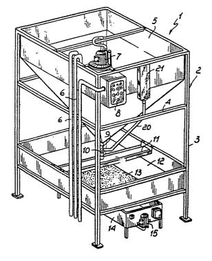
This invention relates to an apparatus for purifying industrial waste water and the like.
