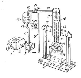
This invention relates to a hydraulic cylinder actuated wood cleaver, the novel feature whereof resides in that it is driven by the engine of a portable chain saw, from which the cutting chain has been removed.
