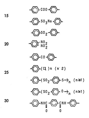
In the stabilized polyphenylene sulfide of the present invention, the aromatic constituents having the electron attractive substituents must be present in the chain ends or branched chains or in the main chain in order to provide the best stabilizing efficiency. A comparable
