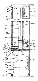
This invention relates to a vending machine which has been designed for vending heated items or articles, and in particular heated items of food, such as hamburgers.
