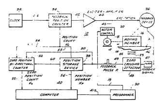
This invention relates generally to electronic control systems for apparatus having movable members, such as machine tools or the like. In particular, it relates to control systems including position monitoring systems for monitoring the position of reversibly movable moving members in such apparatus.
