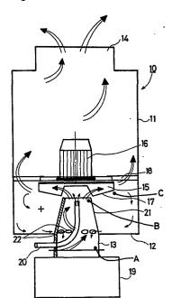
Means for removing gaseous components and/or solid impurities present in a gaseous fluid flow
