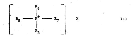
wherein  $R_5$  represents alkyl or alkenyl groups of from 8 to 24 carbon atoms;  $R_6$ ,  $R_7$ , and  $R_8$  represent an alkyl or alkenyl group containing from 1 to 4 carbon atoms; and X is as defined above.
