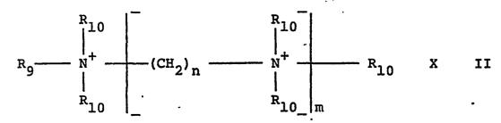
wherein  $R_9$  is an alkyl or alkenyl group of from 8 to 22 carbon atoms, and each  $R_{10}$  independently represents a  $C_1$ - $C_4$  alkyl group -  $(C_2H_40)_pH$ , -  $(C_3H_60)_qH$  or -  $(C_2H_40)_r(C_3H_60)_sH$ ; wherein n is an integer from 2 to 6; m is an integer from 1 to 5; p,q,r,s, are each a number average in the range from 0 to 14, the sum total of p,q,r, and s in the molecule being from 2 to 14, and
