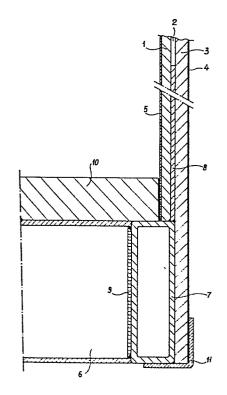
Closed self supporting body for a truck or trailer.
