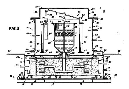
The present invention relates to apparatus for casting of low-density alloys and especially alloys such as magnesium-based alloys which require protection from oxidation during the pouring operation. In particular, 5 the invention relates to apparatus for the casting of such metals into ceramic or sand molds in which the castings are thin walled and consequently difficult to cast because of problems with incomplete filling of the molds.
