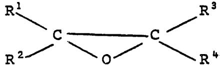
wherein each of  $R^1$ ,  $R^2$ ,  $R^3$  and  $R^4$  is hydrogen or an aliphatic radical or any two thereof together form a cyclic radical, said epoxide containing at least 8 carbon atoms.
