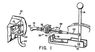
This invention relates to a locking device for an elongate member, such as a cable assembly in a vehicle. Examples of such cable assemblies are transmission cable assemblies and clutch cable assemblies.
