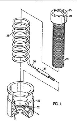
This invention relates to an electricall ? neared ? sprue bushing for injection molding, and more particularly to an improved connector assembly therefor and method of making the same.
