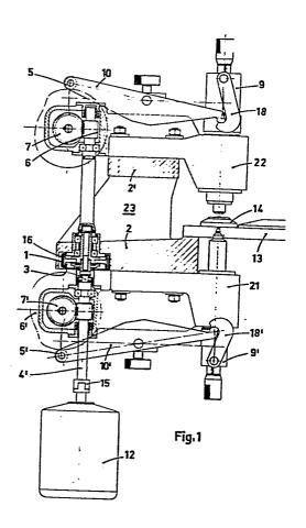
Mechanism for direct transmission of feed movements to the operating units of an automatic machine with revolving table.
