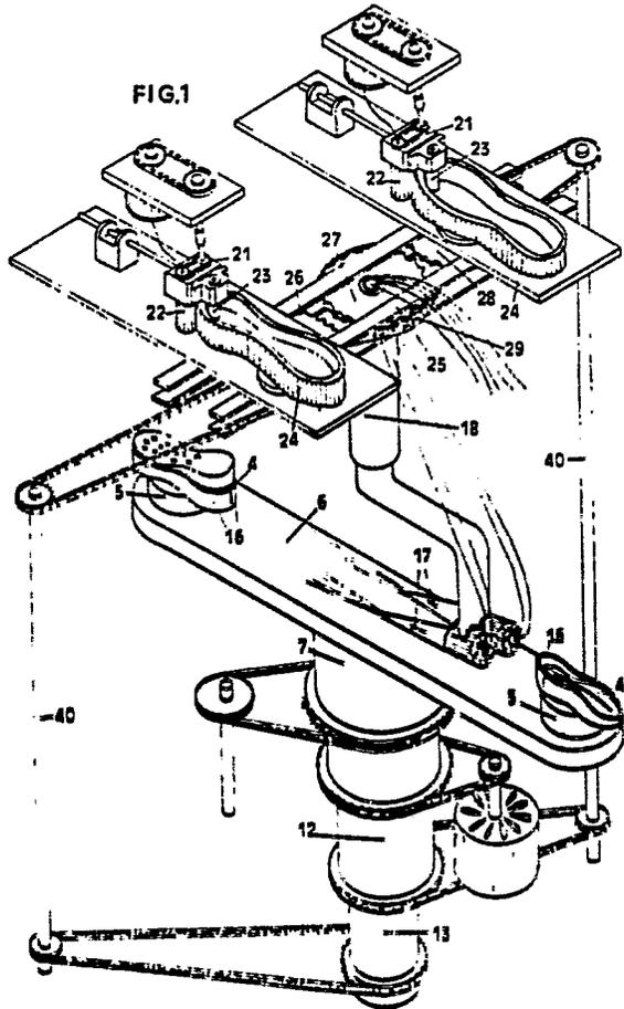
Spraying machine for painting shoe bottoms
