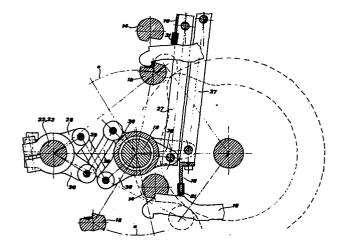
"MEANS FOR CONTROLLING KNIFE OSCILLATIONS AND HOOK MOVEMENTS IN A LOOM DOBBY"
