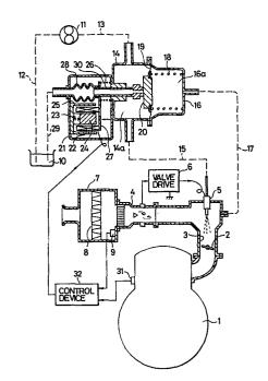
FUEL INJECTION SYSTEM FOR AN INTERNAL COMBUSTION ENGINE, AND AN ENGINE PROVIDED WITH SUCH A SYSTEM
