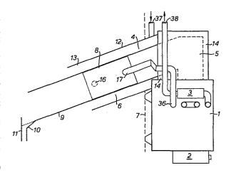
The present invention relates to a fuel-fired heating appliance, particularly to a boiler for heating a circulating fluid as well as to a flue for such an appliance and to a heat exchanger, primarily, but not exclusively, for an appliance of the type defined above.
