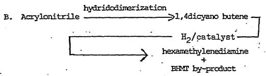
The BHMT by-product is recovered as the bottoms from the distillation of the hydrogenation product in each process. The BHMT by-product, also referred to herein as crude BHMT, typically contains the following components and has the typical Primary Amine Numbers and Base Values indicated below:
