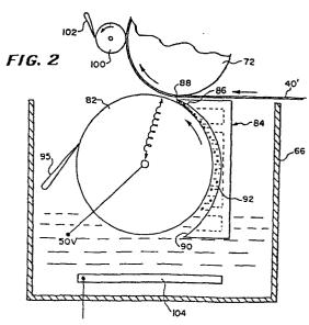
This invention relates generally to the development of latent electrostatic images which are formed on the photoconductive surface of electrophotographic members. More particularly, the invention provides a method and apparatus for effecting such development by transfer rather than using conventional electrophoretic liquid development techniques.
