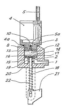
A device for the water feeding and for the filtering of the coffee infusion in coffee-machines particularly of automatic type
