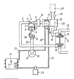
This invention relates to an intake air cooling system for supercharged endothermal engines, in particular engines wherein the intake air is fed through a turbocharger.
