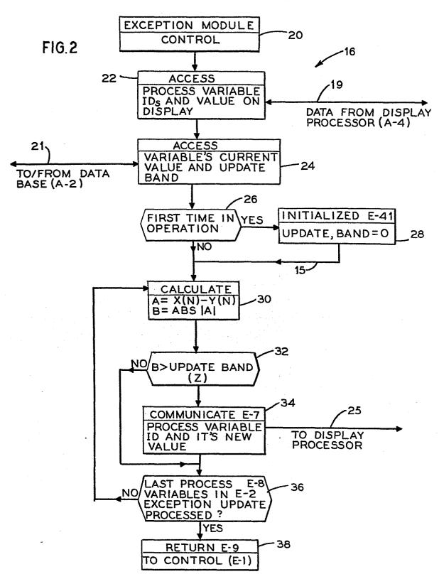
X(N) = PROCESS VARIABLE'S VALUE - NEW FROM DATA BASE Y(N) = PROCESS VARIABLE'S VALUE - ON DISPLAY Z = UPDATE BAND
