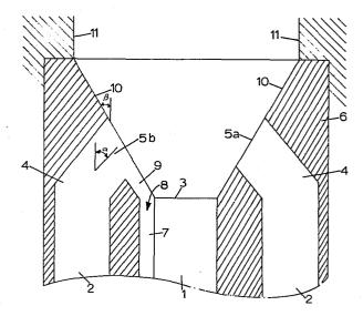
"A ceramic burner for gas, particularly for a hot-blast stove for a blast furnace"
