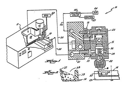
This invention relates to the scaling of closures for containers and particularly to a new apparatus for emplacing seals thereon and to a closure having a seal formed from an adhesive material.
