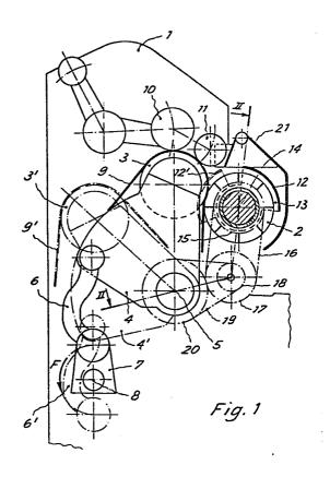
A protecting device for the cylinder with blades in fleshing machines and the like for a tannery, having a movable shield synchronized with the opening of the machine
