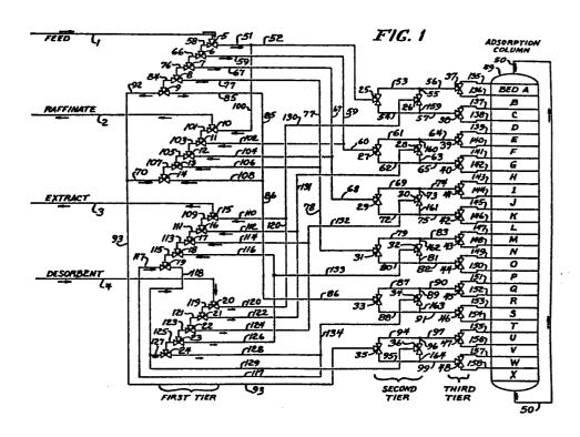
Multiple valve apparatus for performing a fluid-solids contacting process
