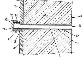
"A method of monitoring the wear of a refractory lining of a metallurgical furnace wall"
