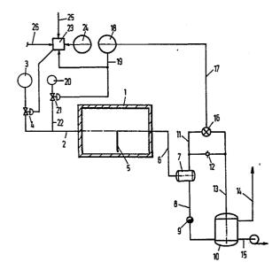
A method and apparatus for removing condensate from a cylinder, in particular a cylinder for drying paper.
