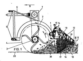
Soil working machine comprising a rotary digging and desintegrating tool and an upearthing device.
