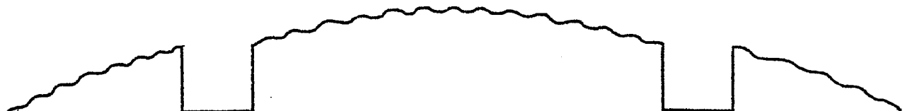
FIG. 1.3 VIDEO SIGNAL WITH SHADING DEFECTS
