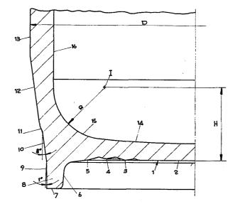
Convex type bottom with a bearing rim for bottles for industrial gases obtained by means of hot forging from a steel billet and fixture for forming said bottom.
